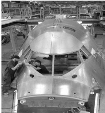
747 cab section manufactured in Wichita
